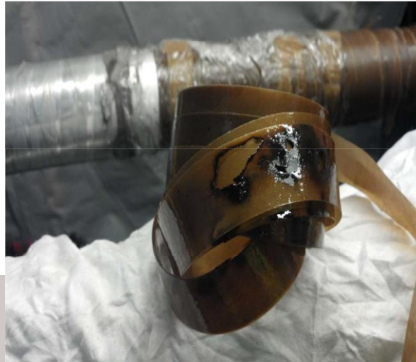
Example of PD in a 138kV HPFF joint (circulated oil)
